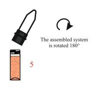
Screw the processing tube II with integrated filter system onto the processing tube I.
